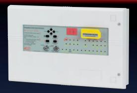
Featuring an intuitive 128 x 64 pixel two-colour graphic display that gives clear and concise feedback to the user, installer and commissioning engineer, the panel also includes six monitored inputs (including hold and abort), a time stamped log, adjustable flood times and volt-free changeover relays for fire, local fire, 1st stage active, 2nd stage active, extractor fan and fault.
