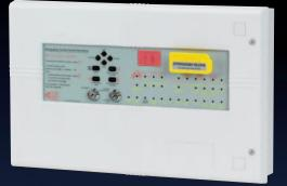
Featuring an intuitive 128 x 64 pixel two-colour graphic display that gives clear and concise feedback to the user, installer and commissioning engineer, the panel also includes six monitored inputs (including hold and abort), a time stamped log, adjustable flood times and volt-free changeover relays for fire, local fire, 1st stage active, 2nd stage active, extractor fan and fault.
