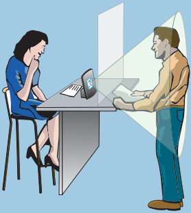
Typical counter loop system using a PL1/K1 portable induction loop kit
