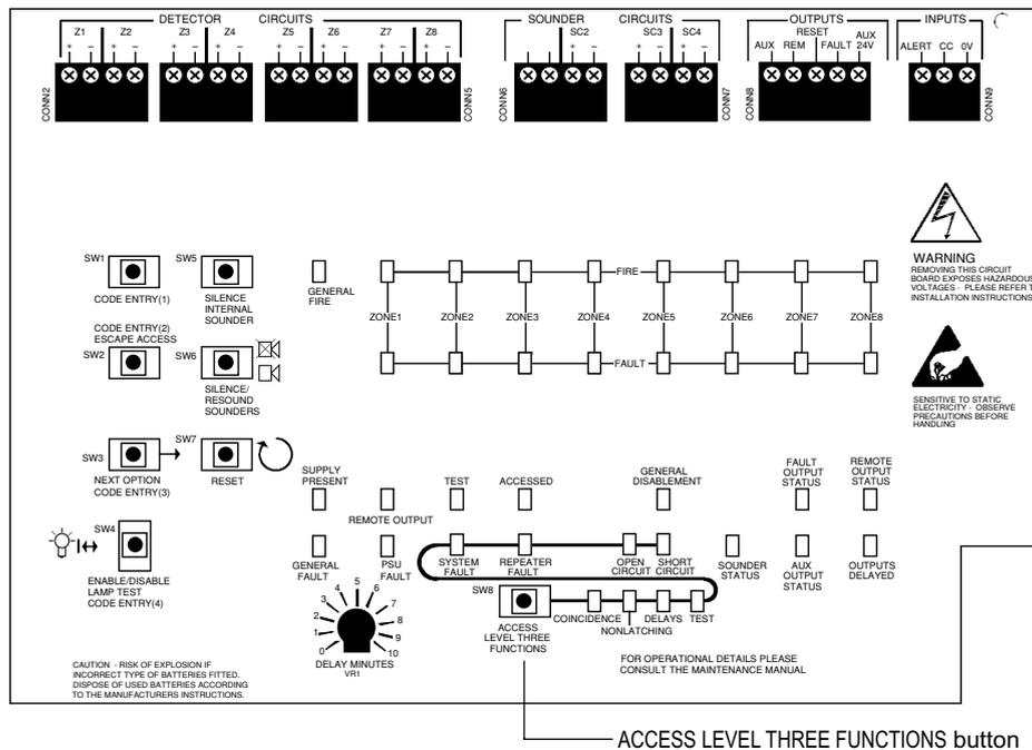
When the ACCESS LEVEL THREE FUNCTIONS button is pressed for the first time, the accessed light will be lit steady, and the Test function will be selected and indicated by its yellow light flashing (see right).
