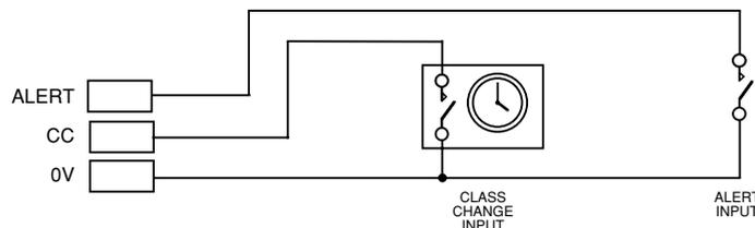
The wiring for each input should be connected to the relevant 5mm connector block on the Main Control PCB and their screens terminated at the panel's base earth post (see page 13 for more details).
