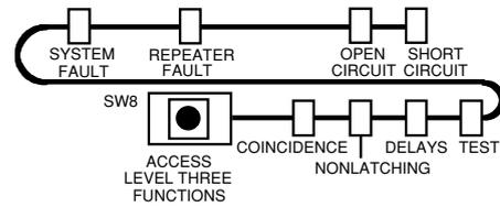
Any existing Zone fault indicators are suppressed and the Zone indicator(s) for any Zone(s) with an open circuit or head out fault are illuminated. For example, if the wiring on Zone 6 is broken or one of its detector heads have been removed, Zone 6's Fault indicator will be lit.
