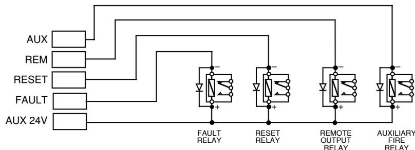
To protect the output stage, only 24V polarised relays with back EMF diodes should be used. If any of the relays are to be used to switch mains potentials, then suitable relays should be chosen and installed and wired accordingly, so as not to compromise the electrical safety of the fire alarm system.
