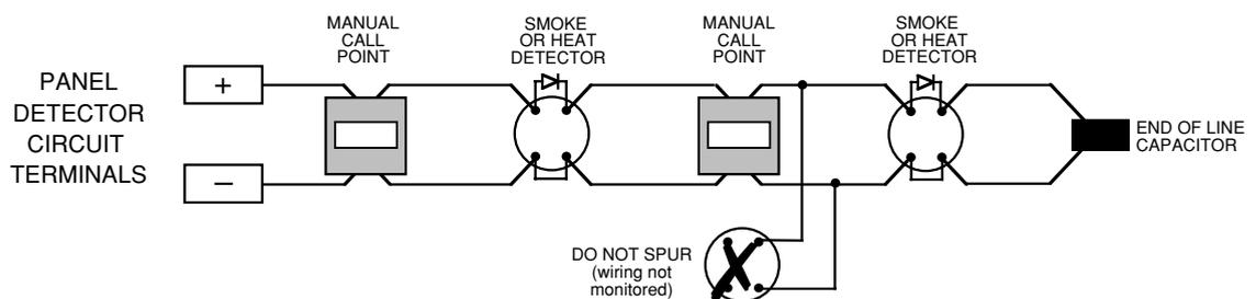
An end of line capacitor (provided in the panel's accessory pack) must be connected across the terminals of the last device on each circuit to allow the wiring to be monitored.
