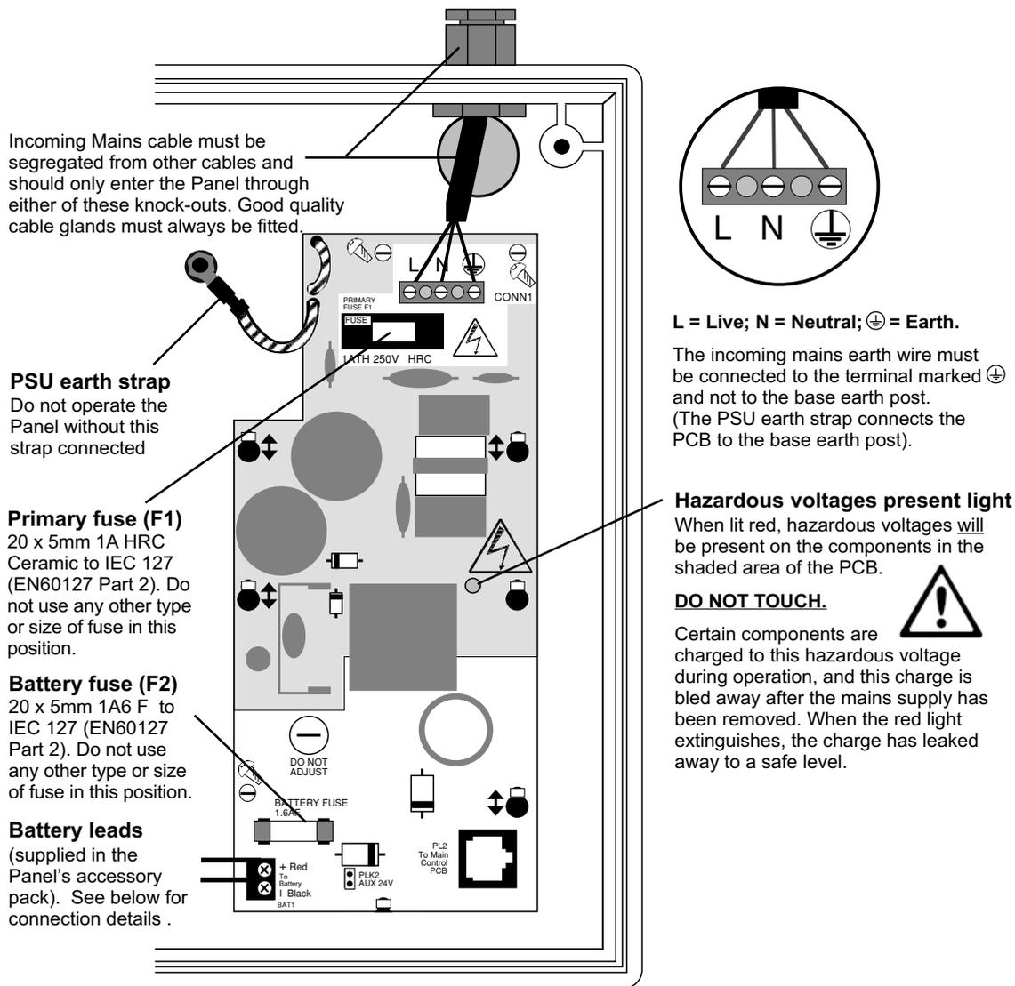
Figure 10 : Battery location and connection details
